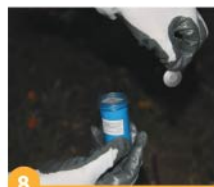
8 Take the igniter powder and metal plate from inside of the box.
